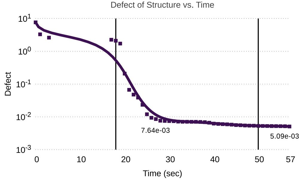
Improvement of structure by algorithm. The three stages of the algorithm are separated by vertical lines. Run on 64 cores.
