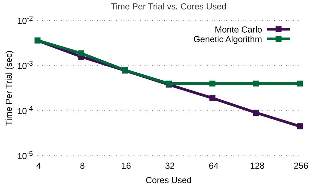
Algorithm speedup from parallelization. Simulations run on the SuperMike-II cluster. Genetic algorithm normalized by trials per "generation" of the algorithm.
