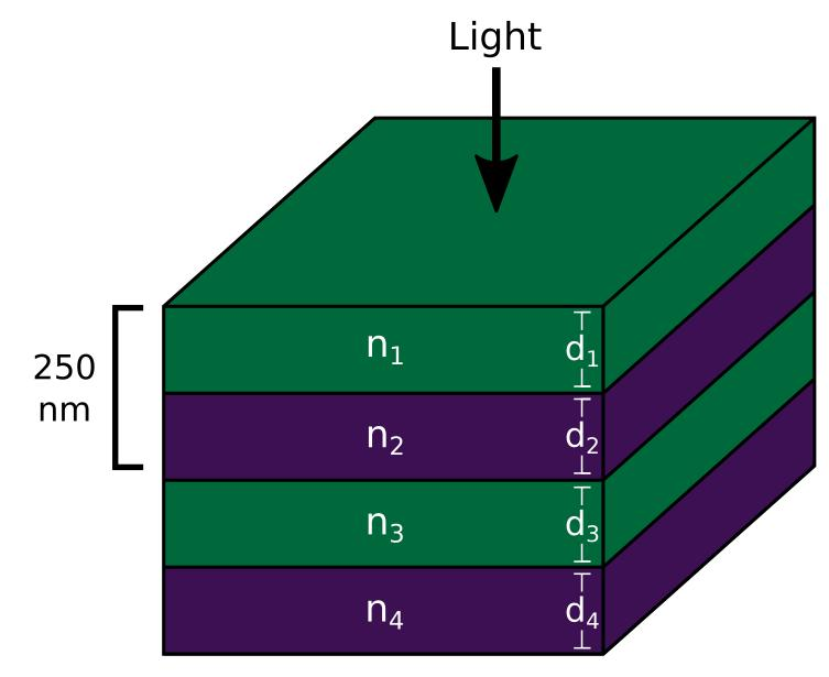
An abstract multilayer thin-film structure. Layer thicknesses and material refractive indices completely characterize a structure.
