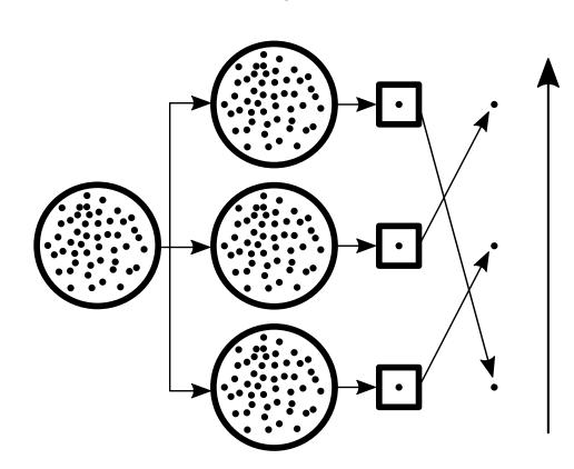
Algorithm flow diagram. First, the best of many randomly generated structures are chosen. Each seeds a "population" with its materials, and thicknesses are optimized. The best of each population is improved, and results are sorted.
