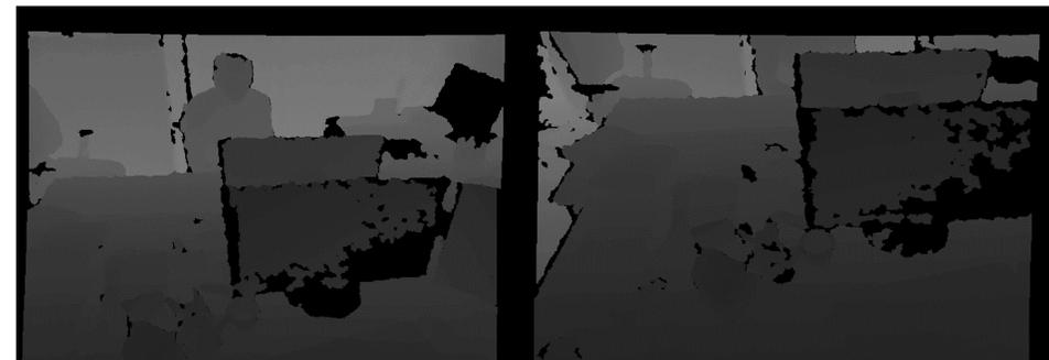
**Figure 4**<sup>2</sup>: The grayscale depth images from the Kinect camera
