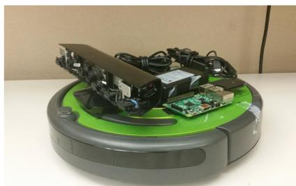
**Figure 2:** The iRobot mounted with the Kinect, which is used to take RGB and depth images.
