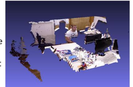
**Figure 6:** The stitched point cloud of the images shown in the "process" section.
