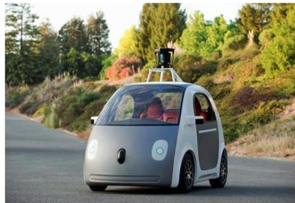
**Figure 1:** The Google Self-Driving Car, which implements advanced SLAM techniques
