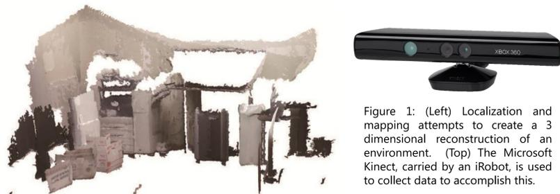
Figure 1: (Left) Localization and mapping attempts to create a 3 dimensional reconstruction of an environment. (Top) The Microsoft Kinect, carried by an iRobot, is used to collect data to accomplish this.
