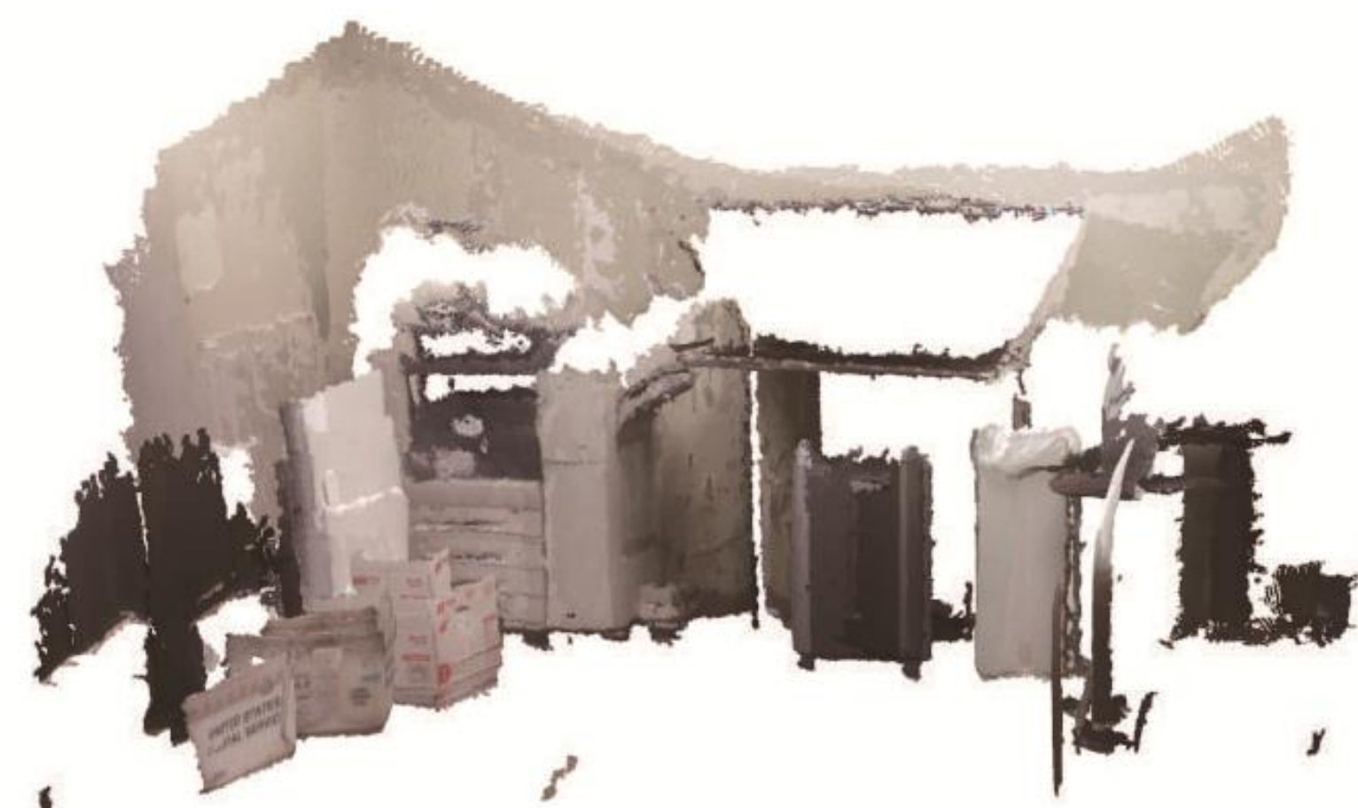
Figure 1: (Left) Localization and mapping attempts to create a 3 dimensional reconstruction of an environment. (Top) The Microsoft Kinect, carried by an iRobot, is used to collect data to accomplish this.
