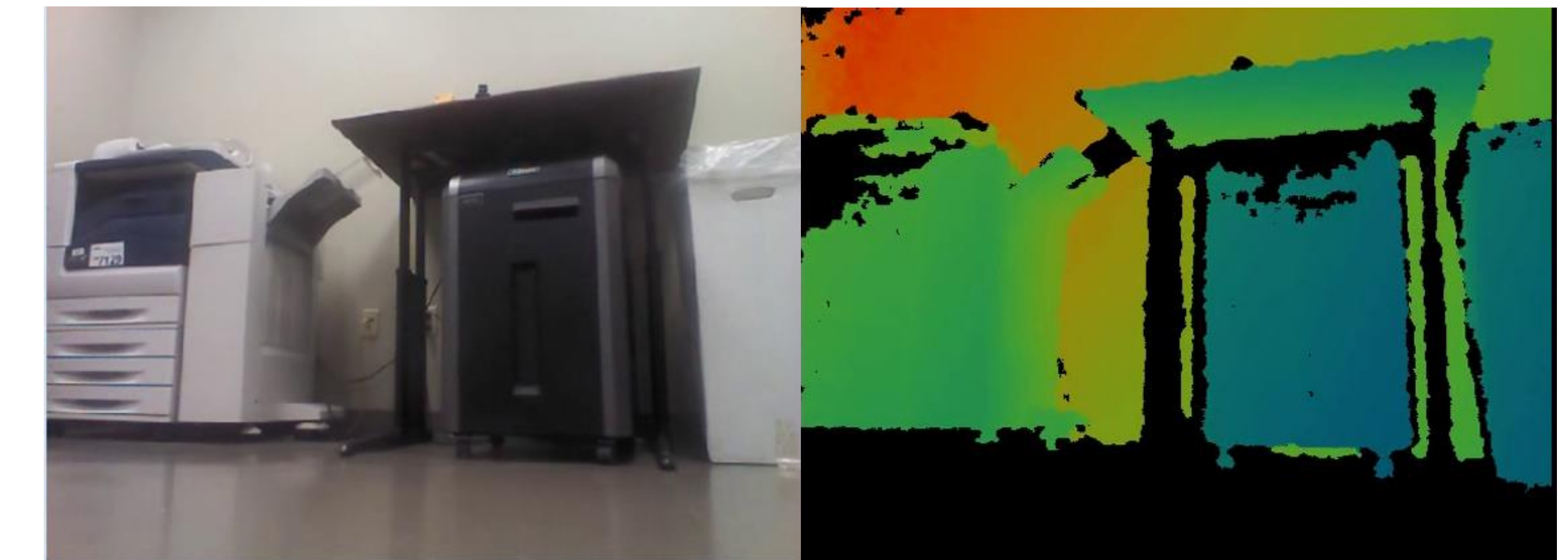
Figure 6: RGB and depth data collected by the Kinect. These are used to progressively reconstruct the environment as demonstrated in Figure 1
