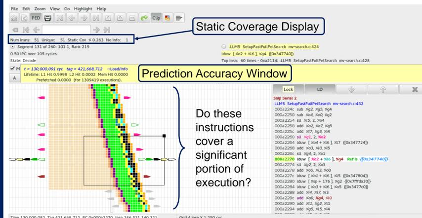
A pipeline execution diagram (PED) plot displays steps and memory addresses for each instruction, with the vertical axis listing single instructions and the horizontal axis measuring clock cycles in the processor. When instructions are found to be incorrect from the result of branch mispredictions, they are restarted for the correct branch and incorrect ones are doomed to be squashed (deleted).
