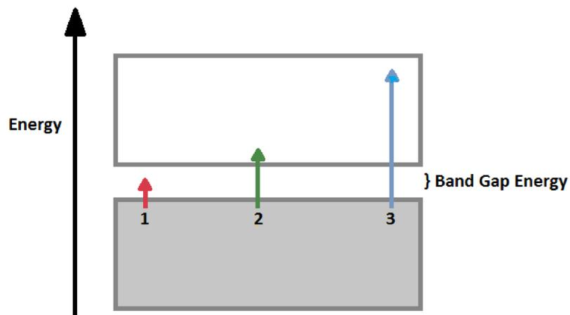
1 – Photons with energy under the BGE (band gap energy) are not able to move electrons to a higher band. Energy from this category of photons is converted into thermal energy.
